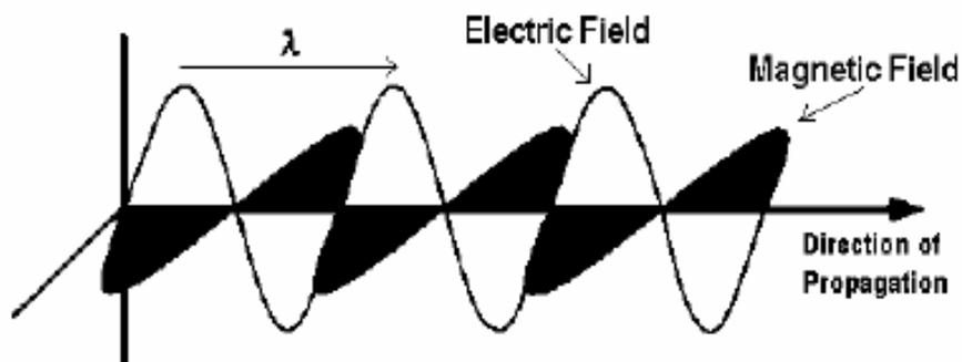
**Figure-1** **Electromagnetic Wave**
