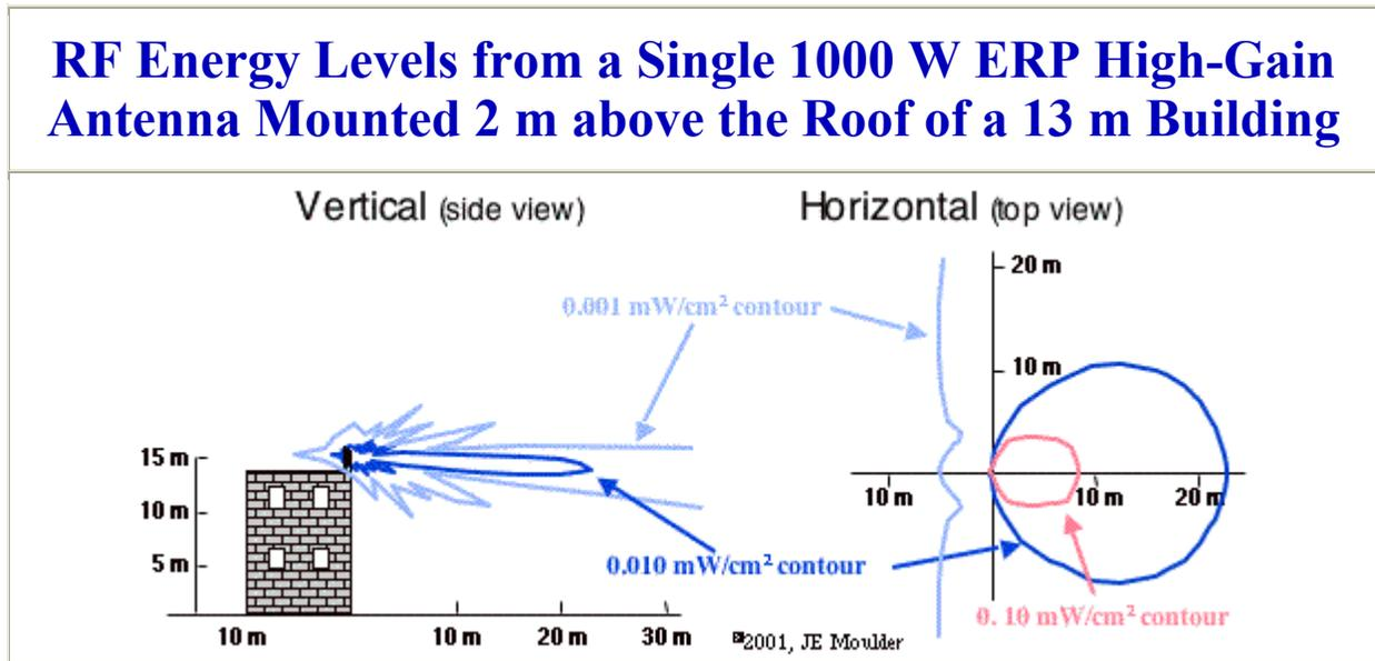
Keep in mind that mobile phone base station that use high-high-gain sector antennas will usually use 3 (or occasionally 4) of these transmission antennas, all pointing in different directions.
